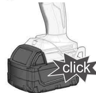
Remove the battery pack before starting any work on the machine.
